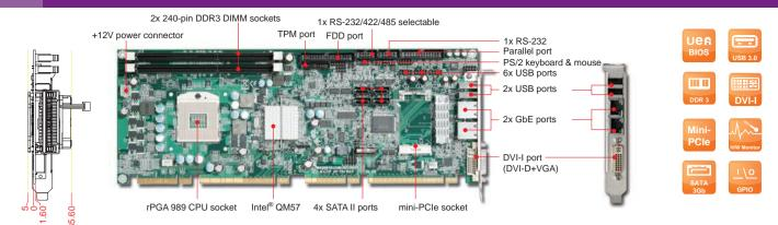
ROBO-8210VG2AR adopts the QM57 chipset and Intel® Core™ i7/i5 and Celeron® processors. Bulit with high performance and lower power consumption than desktop platform, it's suitable for Medical, Industrial Automation and Kiosk applications.
