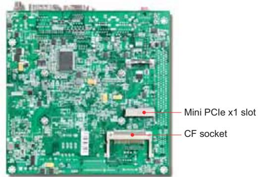
Based on Intel® mobile ICH8M chipset, the WADE-8075/76 takes advantages of Intel® Atom™ D525/N455 technologies. WADE-8075/76 which features low power, is capable of providing dual displays such as LVDS and VGA. In addition, the fanless, low power WADE-8075/76 is the best solution for POS, Medical, Gaming and Digital Signage applications.
