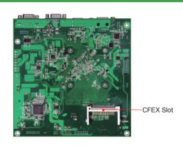
WADE-8078 is the first Portwell off-the-shelf Mini-ITX embedded board product based on the Intel® Atom™ processor E3800 product family with memory and PCI Express controller integrated to support one-channel DDR3L memory and PCI Express 2.0 lanes. Portwell has taken advantage of such technology to furnish a series of products that meets multiple industrial requirements for cost effectiveness, reliable performance and a high level of data integrity and uptime.
